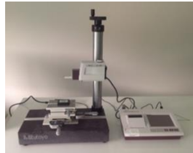
Gambar 3. Roughness Measuring Machine (SJ-411) Mitutoyo
